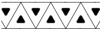
FIG. 6. Schematic picture of antiferrotriatric quasi-long-range order in the triatic phase. Solid triangles represent spin structure of the triatic order formed by three s=1/2 spins on each plaquette.
